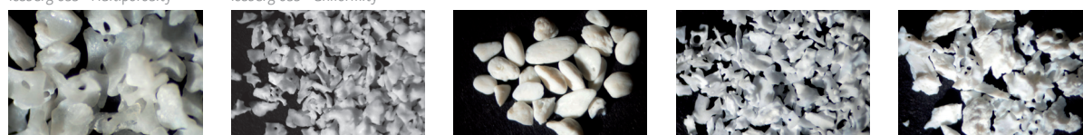
"A" Superficie vitrificada no porosa "A" Nonporous Glassified Surface "A" Porosidad dañada "A" Damaged Porosity "A" Todas las partículas corticales "A" All Cortical Particles "B" No porosa "B" Nonporous Glassified "C" Partícula cortical incluida "C" Cortical Particle Included
